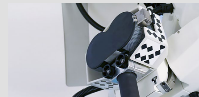
3 DOUBLE COIL ACTIVE/PLACEBO FIXED TO THE ROBOTIC ARM
